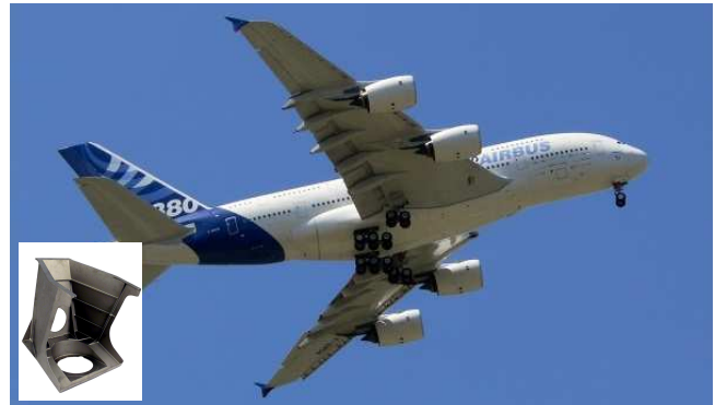
Airbus A 380 with titanium components for the engine pylon.
